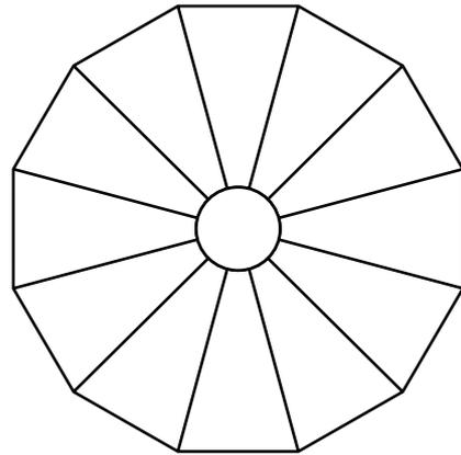
A parachute top is standard. This is constructed from 12 panels that radiate from a centre patch.
