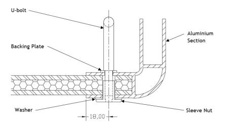
**NOTE:** The U-bolt must  $\underline{not}$  be installed into the honey-comb floor outside of the aluminium edge section.
