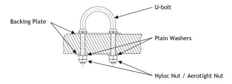
**NOTE:** The U-bolt must  $\underline{not}$  be installed into spreader boards or pilot compartment floors in woven floor baskets.
